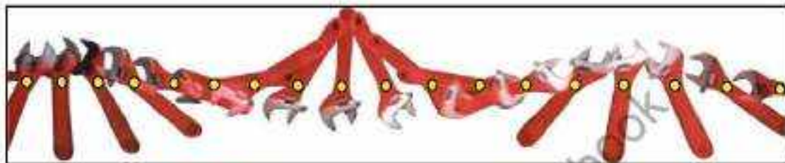
Fig. 4.16: Rotating wrench sliding along a frictionless floor
