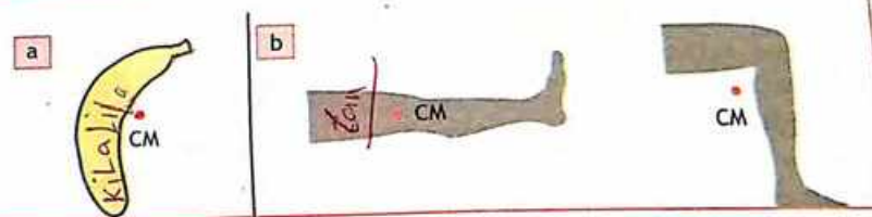
Figure 4.11 CENTER OF MASS OUTSIDE MASS DISTRIBUTION
