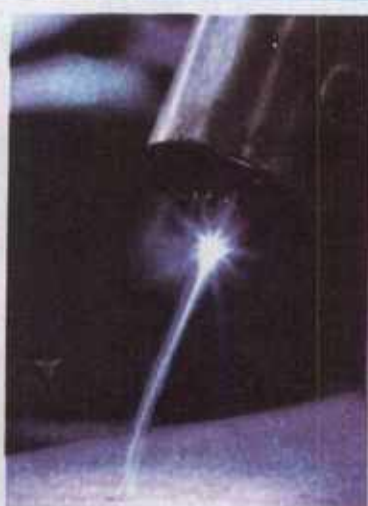
Welding Arc Plasma
