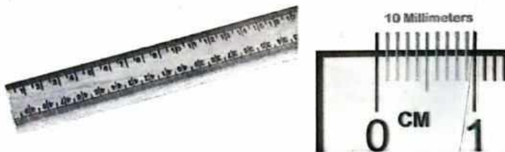
Fig. 8.6: Meter rule and its divisions
