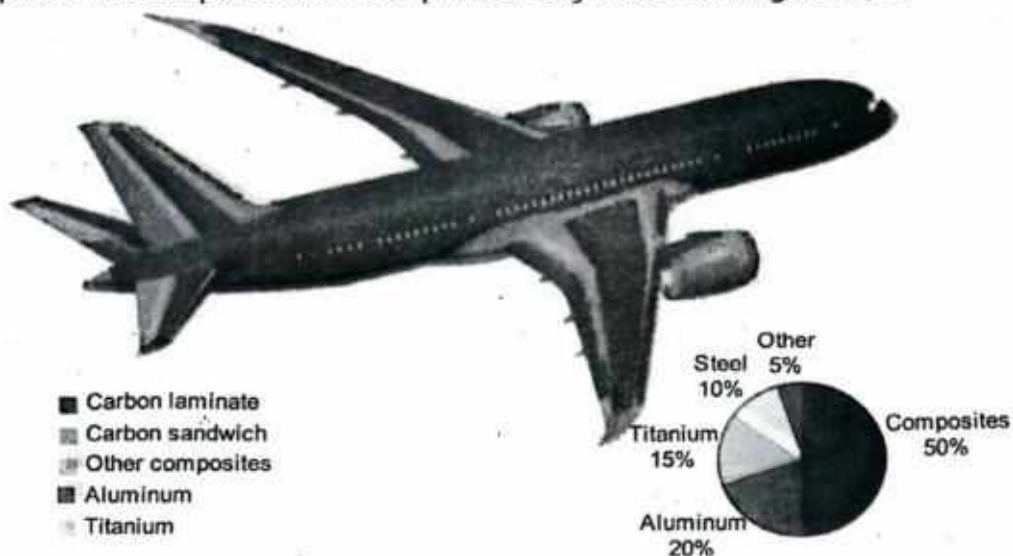
Fig. 7.32: Composition of airplane's body
