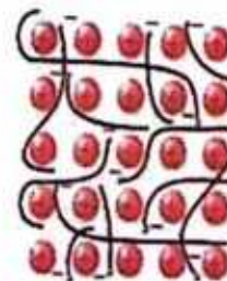
Electrons moving between the cations
