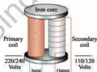
Fig: 16.18 (b) Step down transformer
