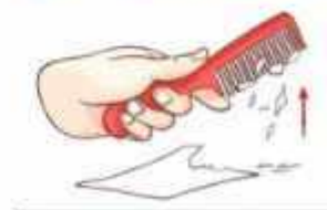
Fig: 14.2 Simple static electric experiment with hair comb.
