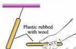
Fig: 14.4 (b) Plastic rods repel each other
