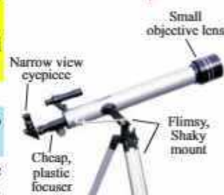
Fig: 13.25. Mechanical parts of a refracting telescope
