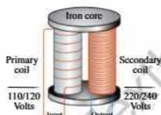
Fig: 16.18 (a) Step up transformer
