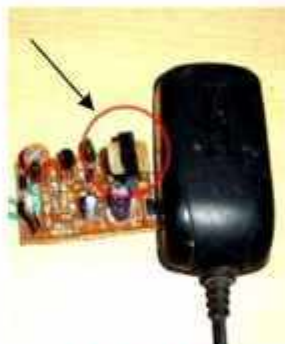
Fig: 16.21 Transformer battery charger
