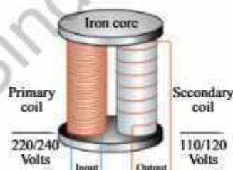
Fig: 16.18 (b) Step down transformer
