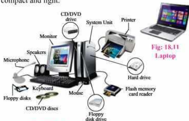
Fig: 18.12. Parts of a computer
