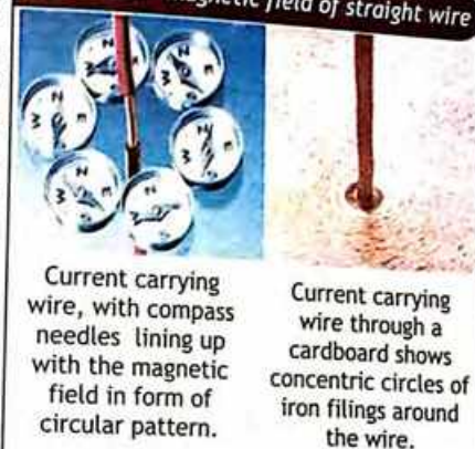
Figure 15.2 - Magnetic field of straight wire
