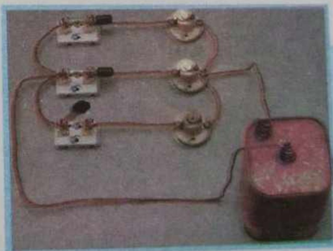
Fig: 6.11 Parallel circuit.
