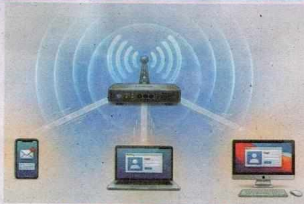
Figure 1.7: Wireless Access Point
