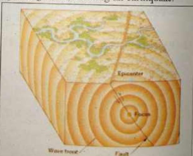
Figure 14.4(a): The focus of an earthquake is the location where rupture begins and energy is released. The place on the surface vertically above the focus is the epicenter. Seismic wave fronts move out in all directions from their source, the focus of an earth.
