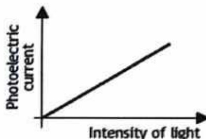
Figure 21.5: Graph of the photoelectric current versus intensity of light.
