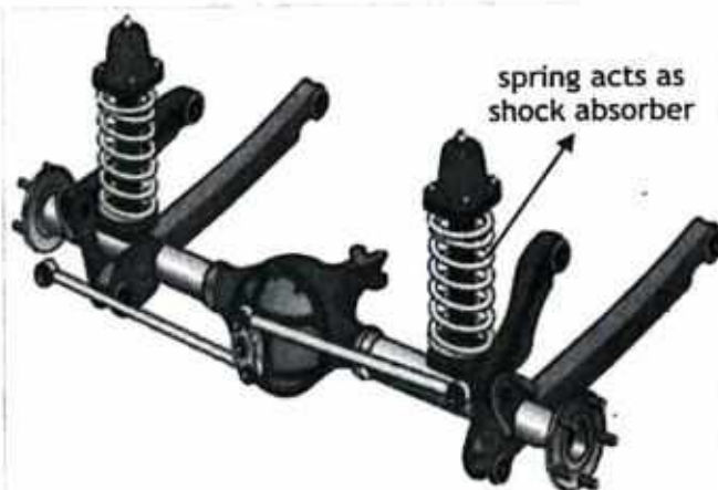
Figure 17.9 (c): Shock absorbers are fluid-filled tubes that turn the simple harmonic motion of the springs into damped harmonic motion.
