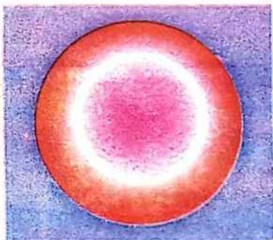
Fig.13.18 A visible circular path of electrons.
