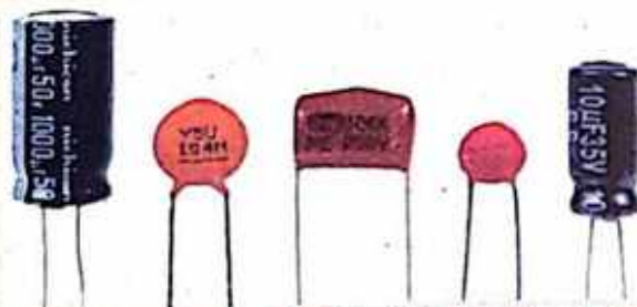
External structure of cylindrical, spherical and parallel plate capacitors.
