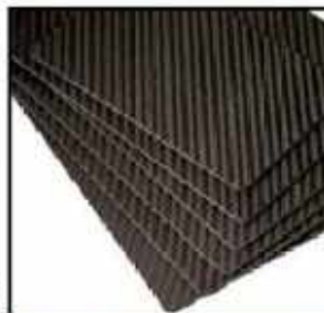
Fig. 9.38: Carbon fibre sheets
