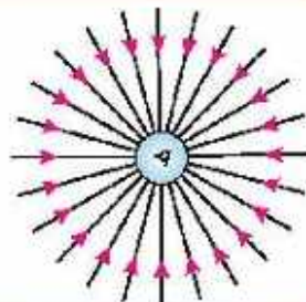
Fig 9.7: The electric field lines are directed radially inward towards a negative point charge -q .
