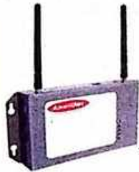
Figure 6.3 Wireless Access Point
